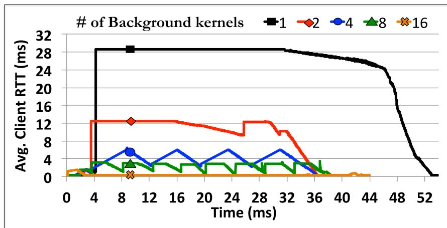
Impact on RTT when running a low-priority background task (BGT) on the same GPU with MemcachedGPU at 4 MRPS. The BGT is split into smaller kernels with fewer CTAs (256 CTAs total). 16 CTAs per BGT kernel reduces the max client *RTT by 18X, while increasing the BGT execution time by 50%.*
