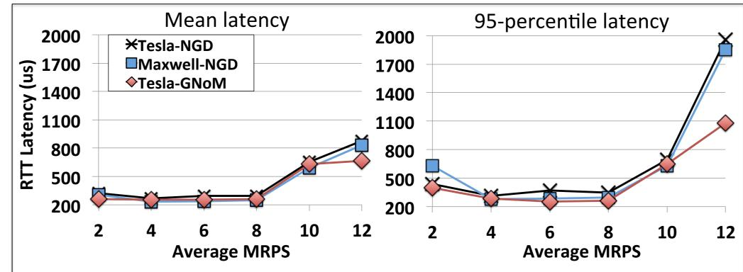
MemcachedGPU Mean and 95-percentile round-trip-time (RTT) latency with 512 requests/batch. GNoM reduces mean latency vs. NGD by 75%-96%.
