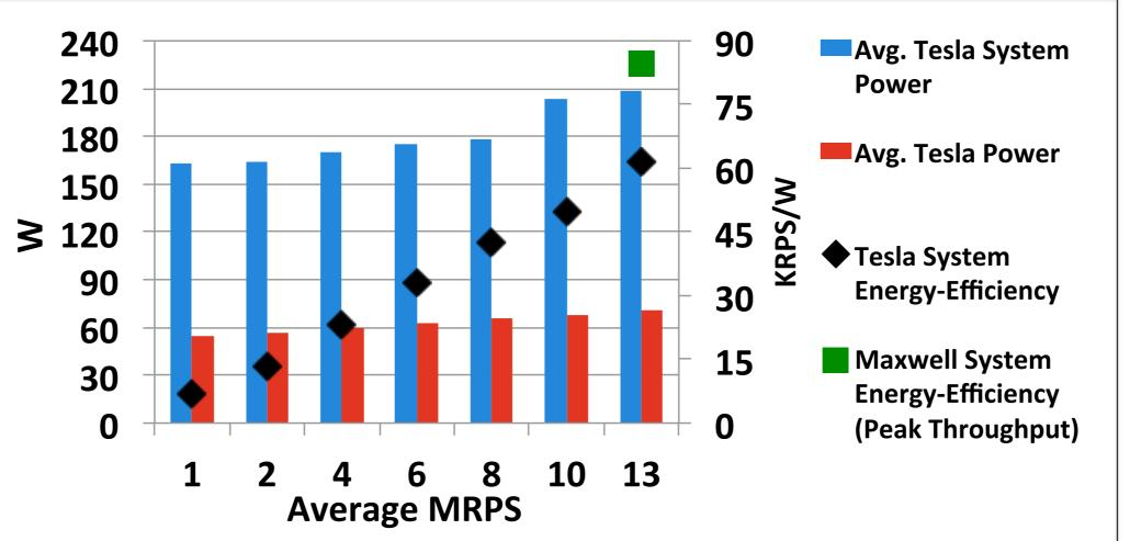
System wall power and energy-efficiency of MemcachedGPU. The Tesla GPU only consumes 32% of peak TDP (underutilizing GPU resources). There are opportunities to further improve total system energy-efficiency through additional GPU I/O and system software support.
