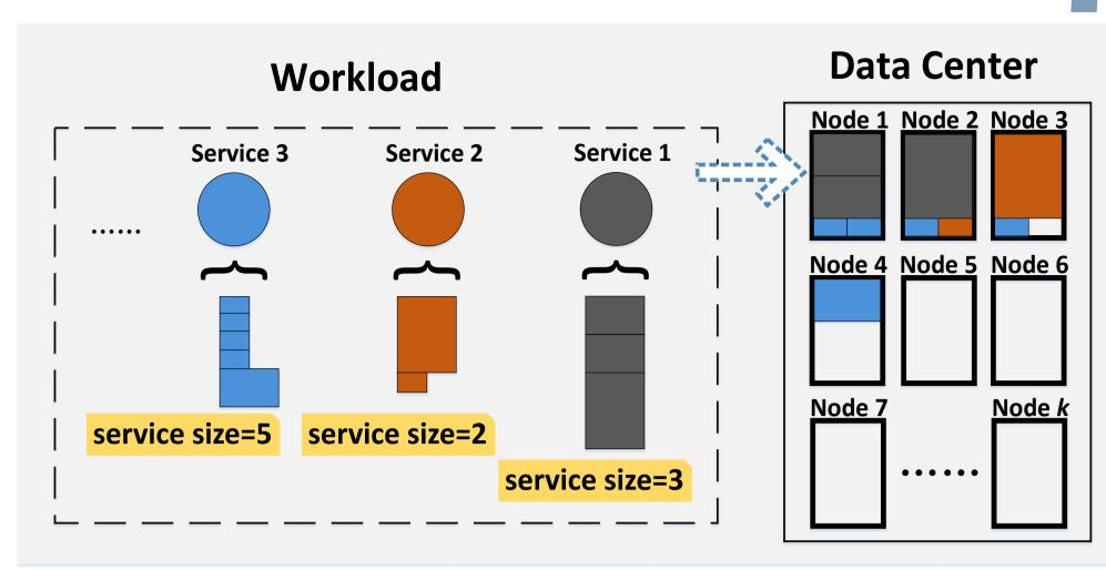
**Resource allocation in the cloud can be seen as bin** packing problem. A *workload* is a sequence of *services*, each of which is constituted of several *instances,* i.e. virtual machines.
